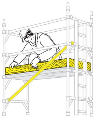
No detail of how toe boards are fitted. Clipped on to uprights on inserted into side boards.
